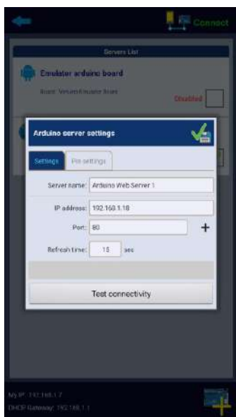
Gambar 6. Arduino setting IP Address
