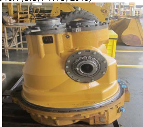
Gambar 2. Component Transmission Condition When Received at Workshop PTTU Banjarmasin
