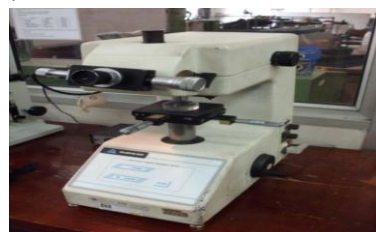
Gambar 8 Alat uji micro hardness tester
