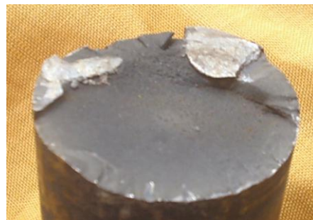
Gambar 1. Permukaan patah poros brine injection pump
