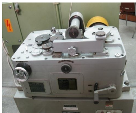
Gambar 10 Alat uji keausan disk on block
