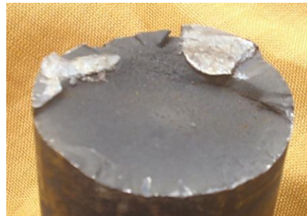
Gambar 1. Permukaan patah poros brine injection pump
