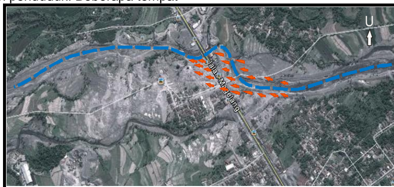
Gambar 4. Arah pelimpasan material akibat lahar di Dusun Gempol, Salam, Magelang. (Anonim, 2012, Google Earth)
