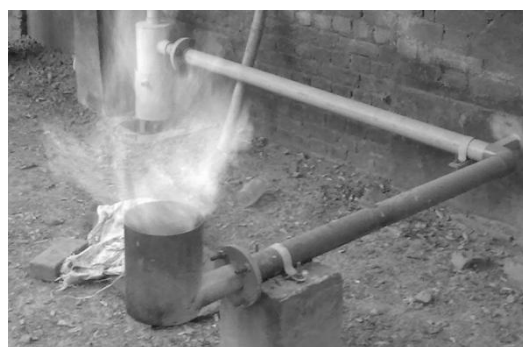
Figure5. Producer gas flame
