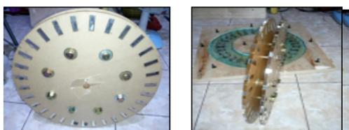
Gambar 4. Rotor generator axial fluks.
