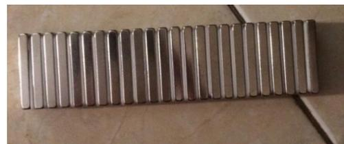
Gambar 2 Magnet permanen neodymium-iron boron/
