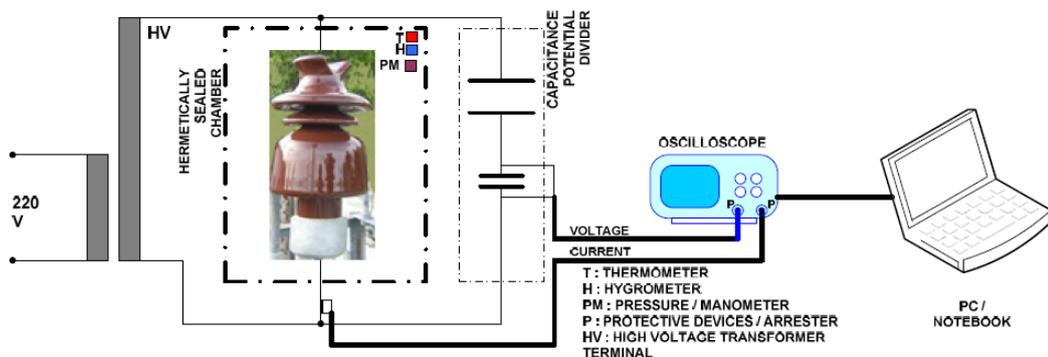
Figure 1. Schematic diagram of experimental setup
