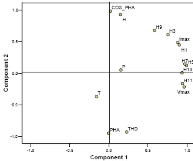
Figure 9. Scatter plot of principal component among parameters on the new-clean porcelain insulator
