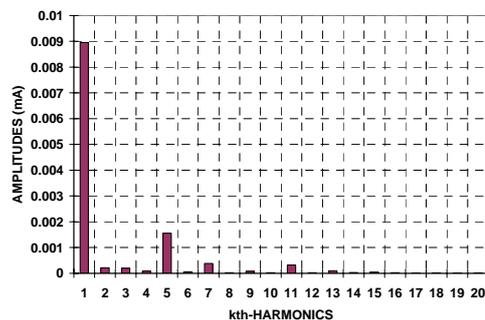
Figure 17. Frequency spectrum of leakage current waveforms of wet new-clean epoxy resin insulator
