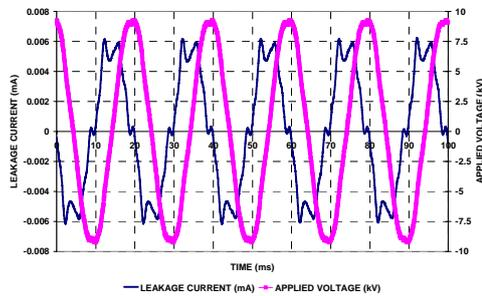
Figure 4. Excel graphical form of applied voltage and leakage current waves of dry new-clean porcelain insulator
