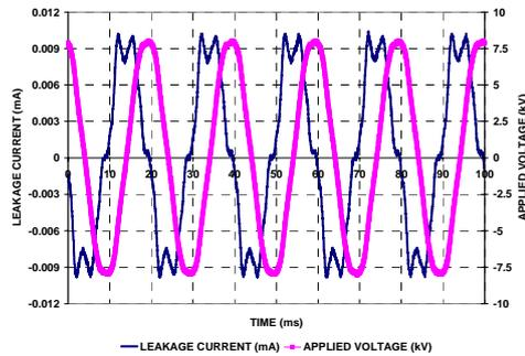
Figure 16. Excel graphical form of applied voltage and leakage current waveforms of wet new-clean epoxy resin insulator
