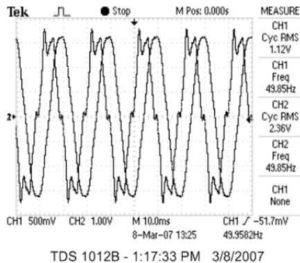
Figure 12. Bitmap form of applied voltage and leakage current waves of dry new-clean epoxy resin insulator
