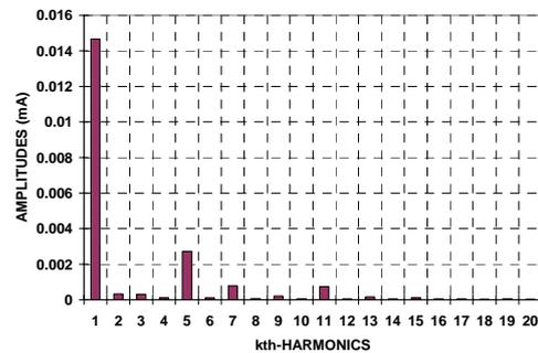
Figure 14. Frequency spectrum of leakage current waveforms of Figure 13
