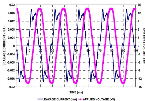
Figure 13. Excel graphical form of applied voltage and leakage current waves of dry new-clean epoxy resin insulator
