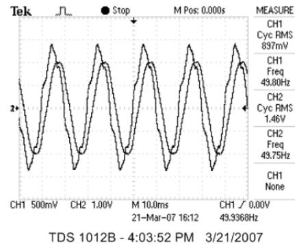
Figure 6. Bitmap form of applied voltage and leakage current waveforms of wet new-clean porcelain insulator
