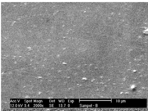
Figure 11. SEM test result of new-clean porcelain insulator specimen
