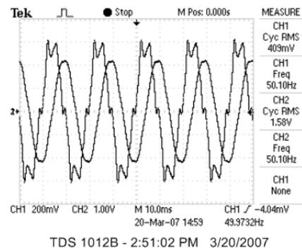
Figure 3. Bitmap form of applied voltage and leakage current waves of dry new-clean porcelain insulator
