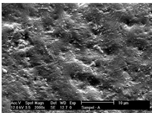
Figure 20. SEM test result of new-clean epoxy resin insulator specimen
