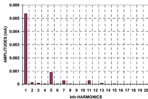
Figure 5. Frequency spectrum of leakage current waveforms of Figure 4
