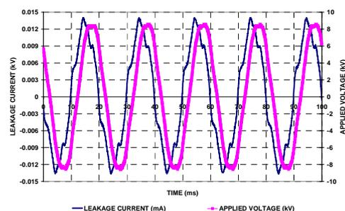
Figure 7. Excel graphical form of applied voltage and leakage current waveforms of wet new-clean porcelain insulator
