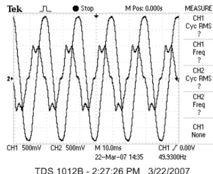
Figure 15. Bitmap form of applied voltage and leakage current waveforms of wet new-clean epoxy resin insulator
