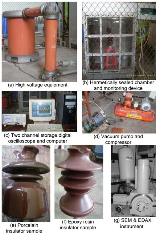
Figure 2. Main experimental equipments
