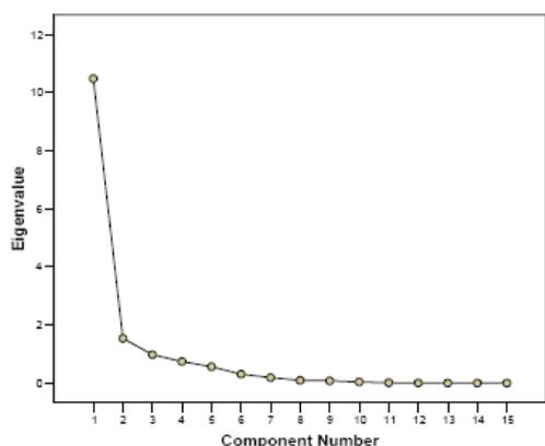
Figure 19. Scree plot of principal component among parameters on the new-clean epoxy resin insulator.
