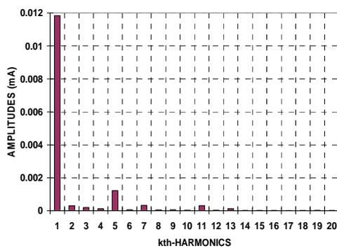
Figure 8. Frequency spectrum of leakage current waveforms of wet new-clean epoxy resin insulator
