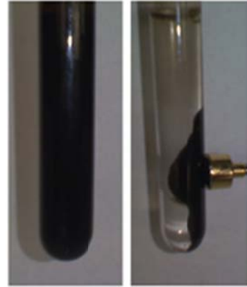
Figure 2. Black precipitation attracted by a permanent magnet.
