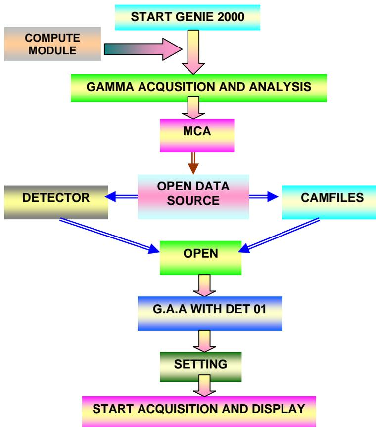
Figure 2. The systematic sketch of Genie 2000 program is operated by MCA and computer system.
