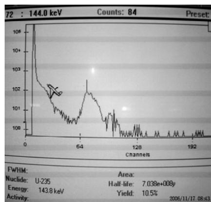
Figure 4. Radiation spectrum on sample 7b (Spl.7b.CNF)
