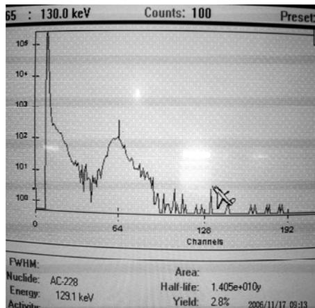
Figure 7. Radiation spectrum on sample 10d (Spl.10d.CNF)
