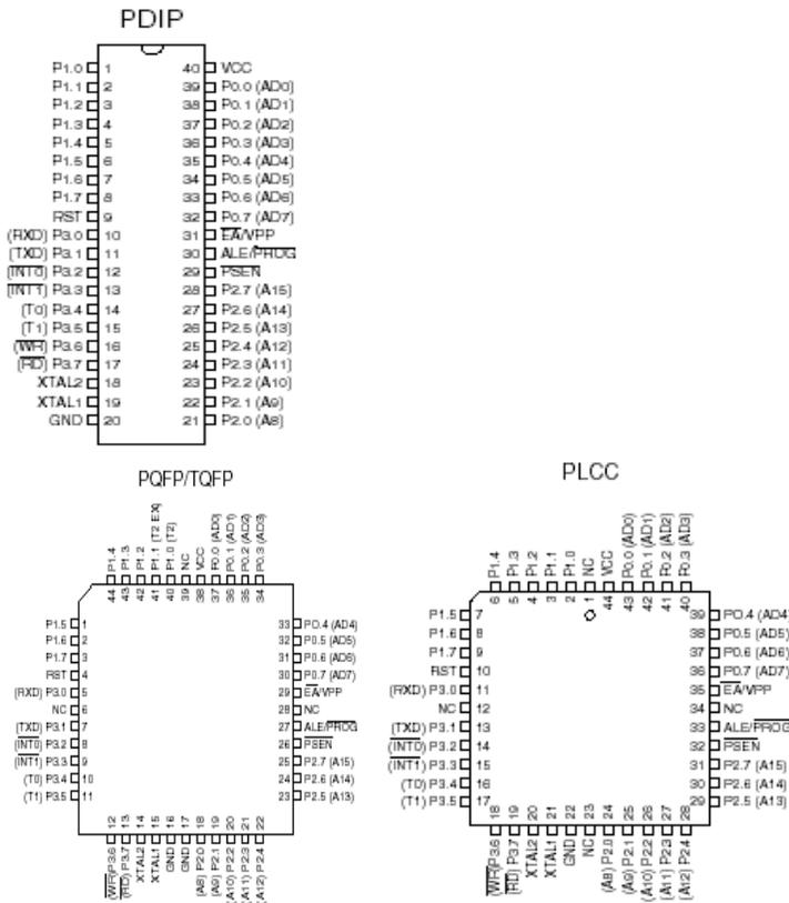
Figure 5 Three model and configuration of AT89C51 Microcontroller
