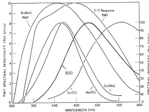
Figure 3 Emission Spectrum of inorganic Scintillators
