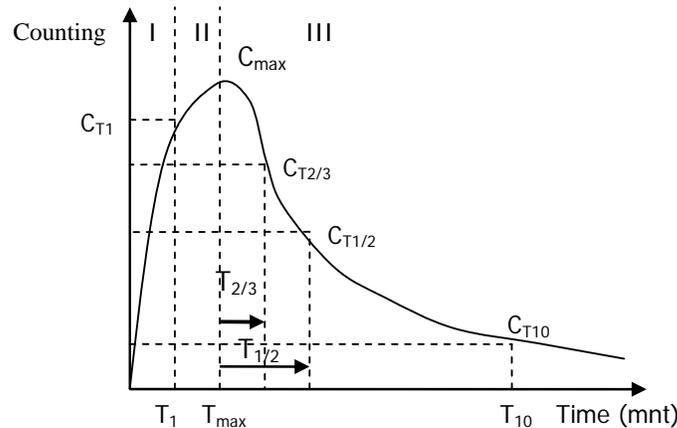
Figure 2 Parameter definition in Renogram Curve Analysis
