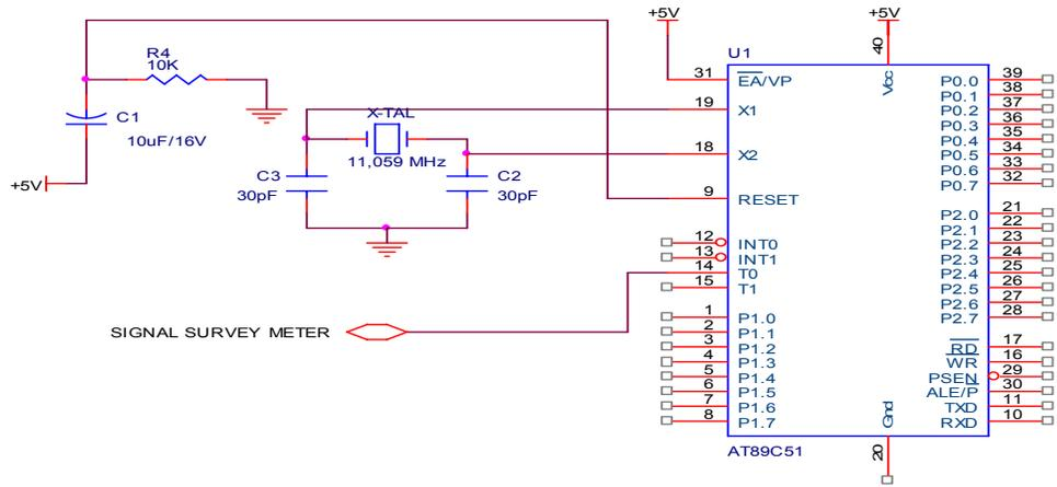
Figure 7 Counter Circuit
