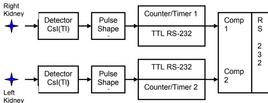
Figure 6 Block Diagram of Renograph with CsI(Tl) Detector and AT89C51 Microcontroller
