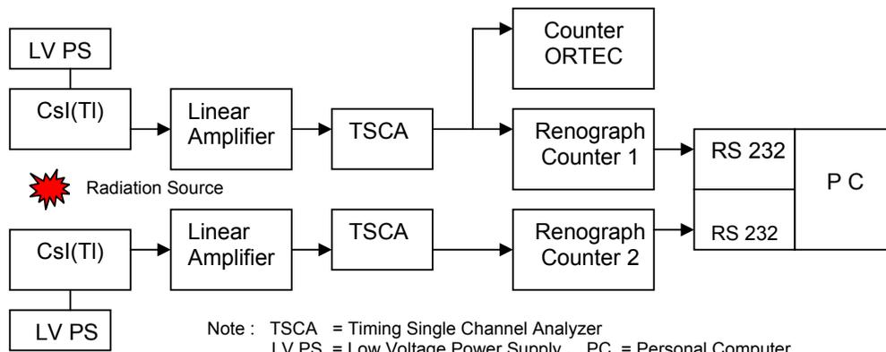
B. Dynamic Testing with radioactive source
