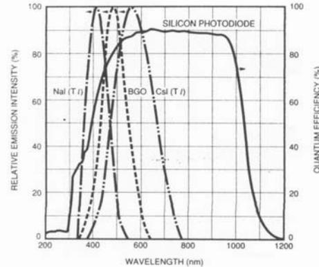
Figure 4 Spectrum respon of Hamamatsu Photo diode S3590-08 and emission spectrum of Scintillators
