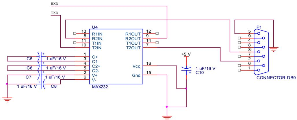
Figure 8 TTL-RS232 Converter Circuit
