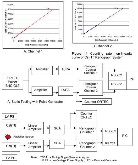
B. Dynamic Testing with radioactive source
