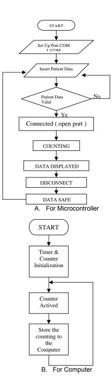
Figure 9 Flow Chart of Program on Microcontroller and Computer System
