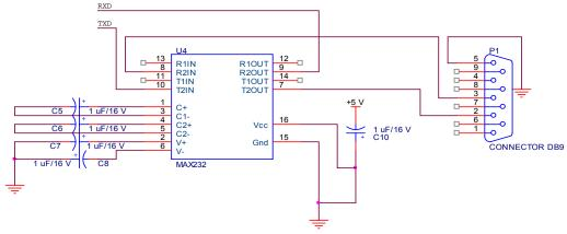
Figure 8 TTL-RS232 Converter Circuit
