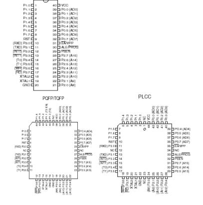
Figure 5 Three model and configuration of AT89C51 Microcontroller
