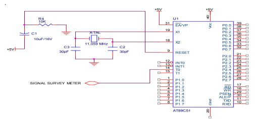
Figure 7 Counter Circuit
