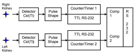
Figure 6 Block Diagram of Renograph with CsI(TI) Detector and AT89C51 Microcontroller
