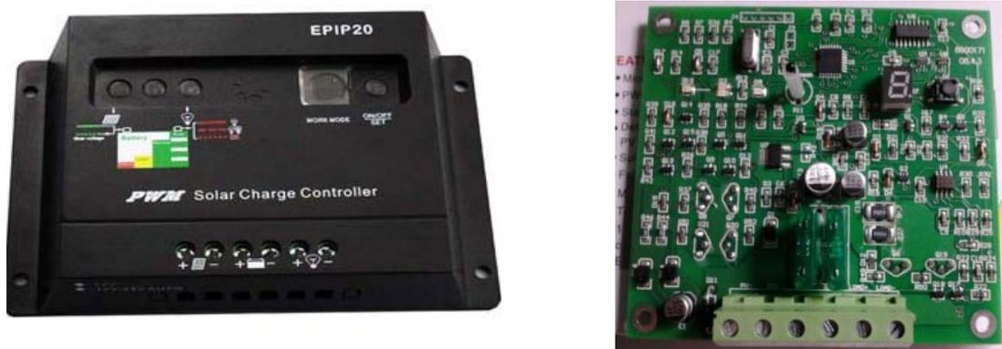
Gambar 3. Solar Charge Controller
