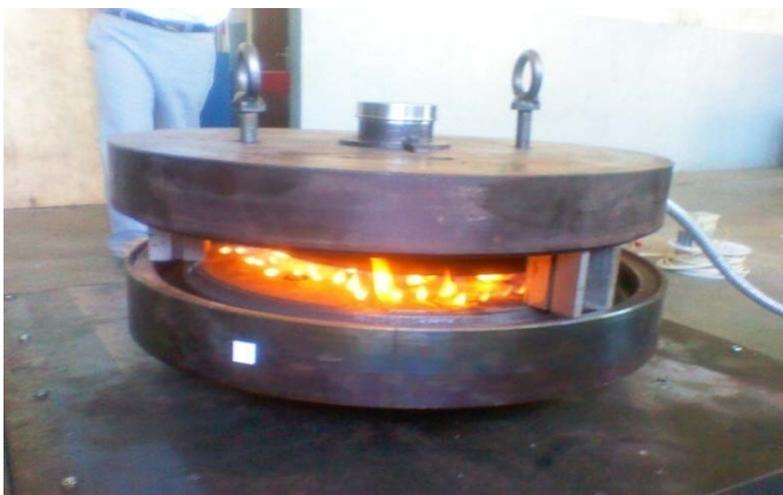
**Gambar 1.** Alat centrifugal casting (Bambang, U, 2010)
