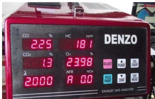
Gambar 4. *Exhaust Gas Analyzer*
