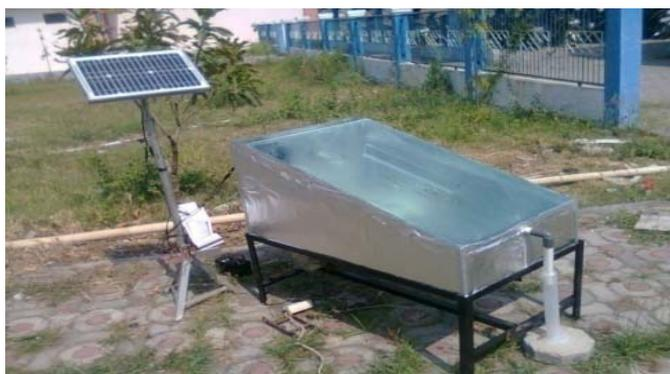
Gambar 4. Alat Hibrid Solar Distilasi
