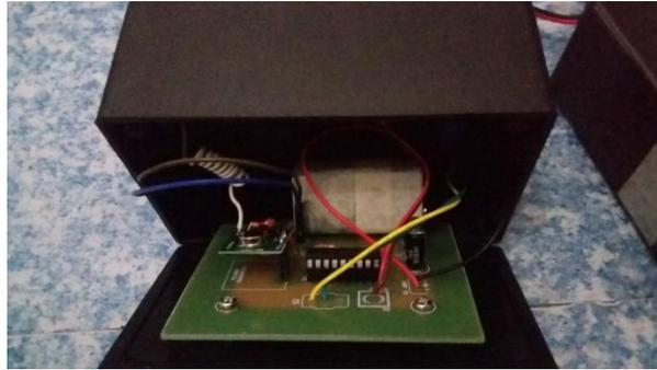
**Gambar 7.** Rangkaian Pengendali RF *Transmitter*
