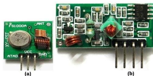
**Gambar 1.** Modul RF XD FST FS1000A (a) *Transmitter* (b) *Receiver*
