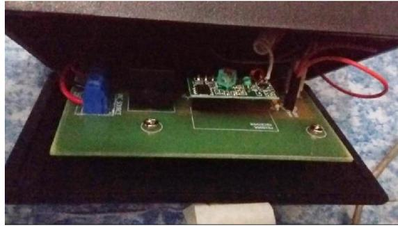
**Gambar 8.** Rangkaian Pengendali RF Receiver
