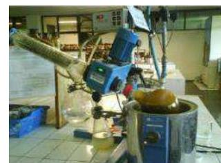
Gambar 2 Vacum Rotary evaporator
