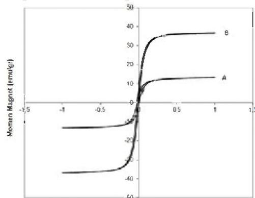
**Figure 8.** Magnetic hysteresis loops taken at room temperature of iron sand coast (A) Raw material magnetic particle attracted to permanent magnet, (B) magnetic particle size <+212  $\mu\text{m}$ , The highest percentage dominated by magnetite (black)
