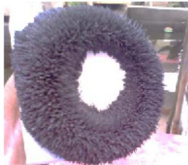
**Figure 4.** iron sands attracted to permanent magnet.
