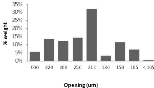
**Figure 6.** The average distribution of sand grain size of magnetic sand
