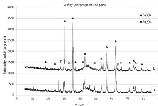
**Figure 9.** XRD pattern indicate that Fe<sub>3</sub>O<sub>4</sub> (magnetite) and  $\gamma$ -Fe<sub>2</sub>O<sub>3</sub> (maghemite)
