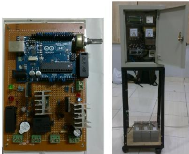
Gambar 10 . Rangkaian Charge Controller
