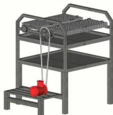
Gambar 2. Desain Alat Bakar Daging Otomatis 3D
