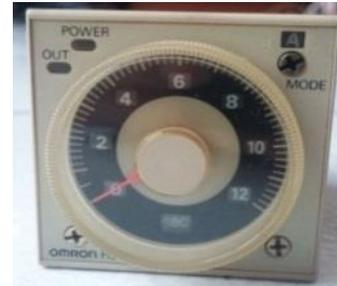
Gambar 2. Timerdelay relay
