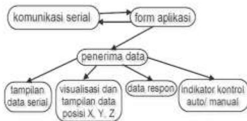
Gambar 8. Blok diagram *ground segment*
