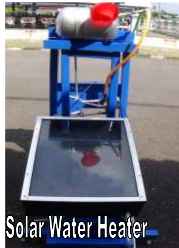
Gambar 7. Solar Water Heater
