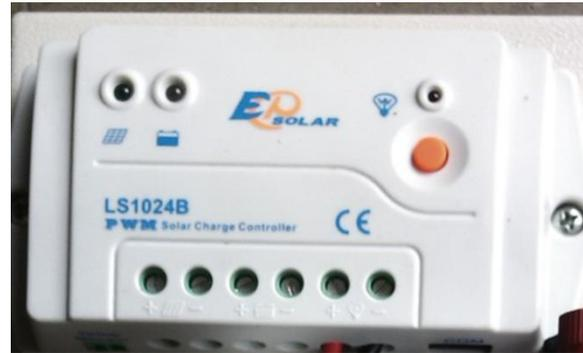
Gambar 5. Contoh Solar Charger Controller
