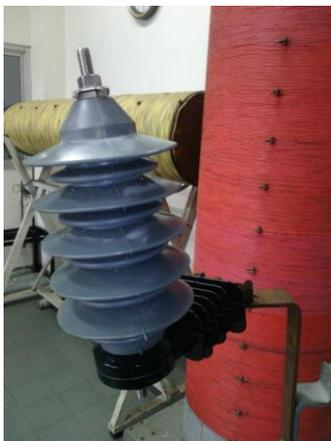
Gambar 5 *Lightning Arrester* tipe ZnO
