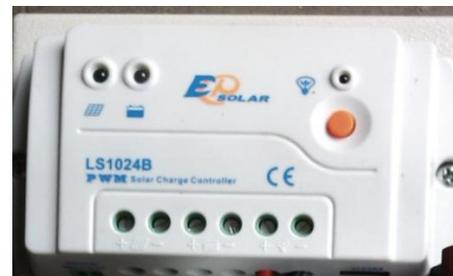
Gambar 5. Contoh Solar Charger Controller
