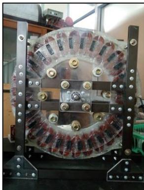
Gambar 7. Generator Axial Fluks.
