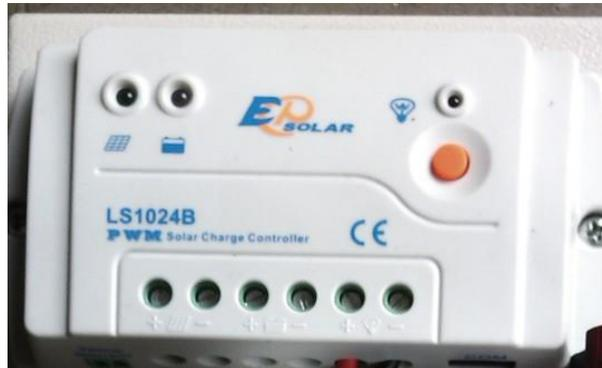
Gambar 6. Contoh Solar Charger Controller
